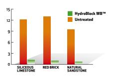
The graph above shows the visible effect HydroBlock  $WB^{TM}$  has on reducing the water absorption of various materials.
